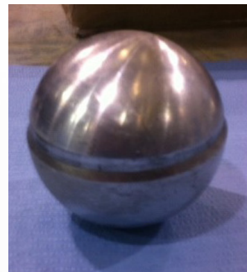
Fixture is removed from test cell and disassembled noting ball extrusion.
