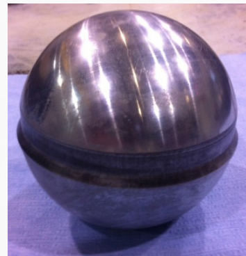
Fixture is removed from test cell and disassembled noting ball extrusion.
